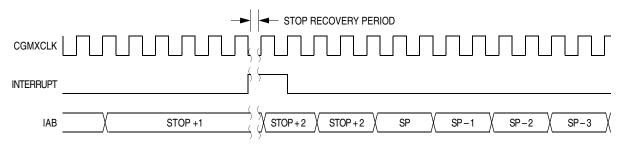
Figure 14-17. Stop Mode Recovery from Interrupt
