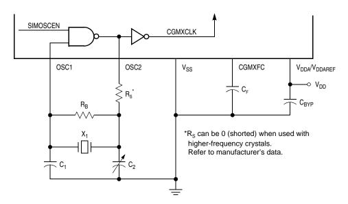
Figure 5-3. CGM External Connections
