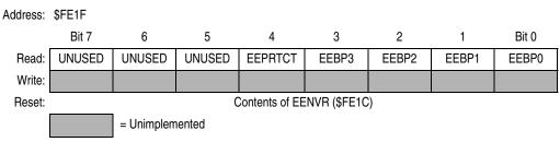
Figure 2-4. EEPROM Array Configuration Register (EEACR)
