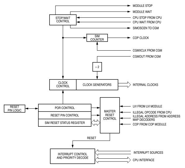
Figure 14-2. SIM Block Diagram
