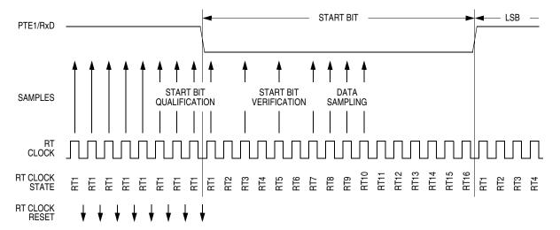
Figure 13-7. Receiver Data Sampling
