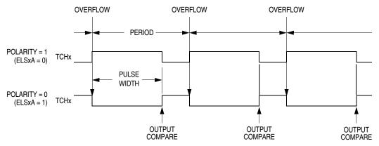
Figure 16-4. PWM Period and Pulse Width
