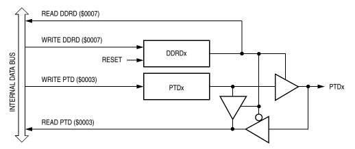
Figure 12-13. Port D I/O Circuit
