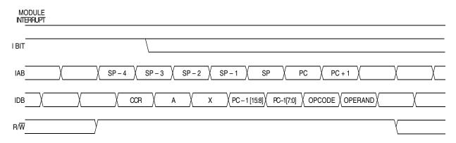
Figure 14-10. Hardware Interrupt Recovery
