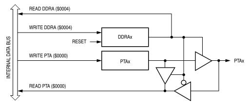
Figure 12-4. Port A I/O Circuit
