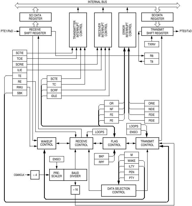
Figure 13-3. SCI Module Block Diagram
