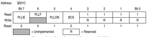
Figure 5-4. PLL Control Register (PCTL)
