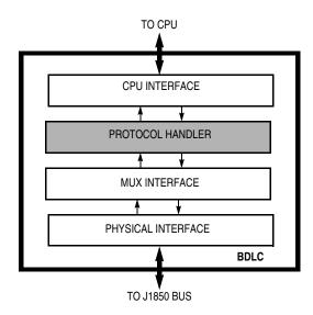
Figure 4-14. BDLC Block Diagram
