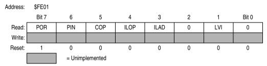
Figure 14-19. SIM Reset Status Register (SRSR)
