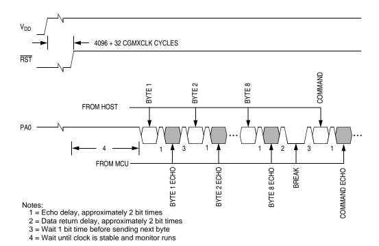
Figure 17-13. Monitor Mode Entry Timing
