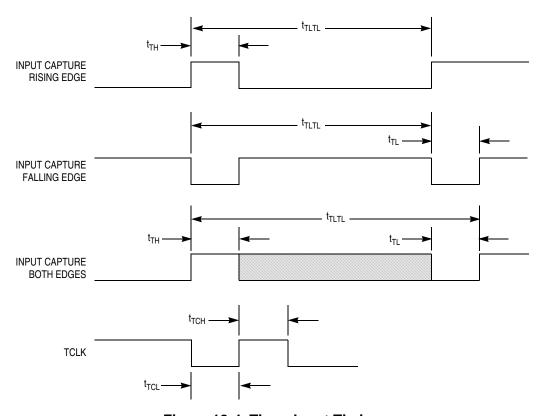
Figure 18-4. Timer Input Timing
