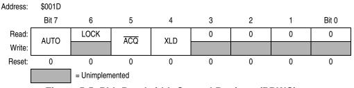
Figure 5-5. PLL Bandwidth Control Register (PBWC)
