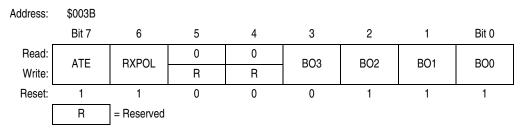
Figure 4-17. BDLC Analog and Roundtrip Delay Register (BARD)
