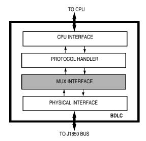
Figure 4-5. BDLC Block Diagram
