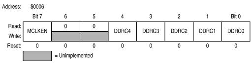
Figure 12-9. Data Direction Register C (DDRC)
