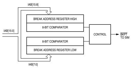
Figure 17-1. Break Module Block Diagram
