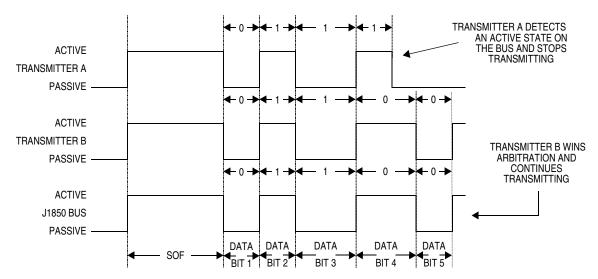
Figure 4-13. J1850 VPW Bitwise Arbitrations
