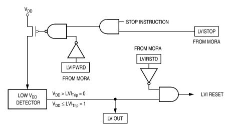
Figure 9-1. LVI Module Block Diagram
