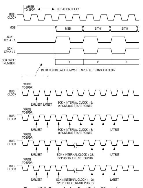
Figure 15-8. Transmission Start Delay (Master)
