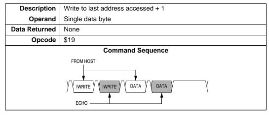
A sequence of IREAD or IWRITE commands can access a block of memory sequentially over the full 64-Kbyte memory map.
