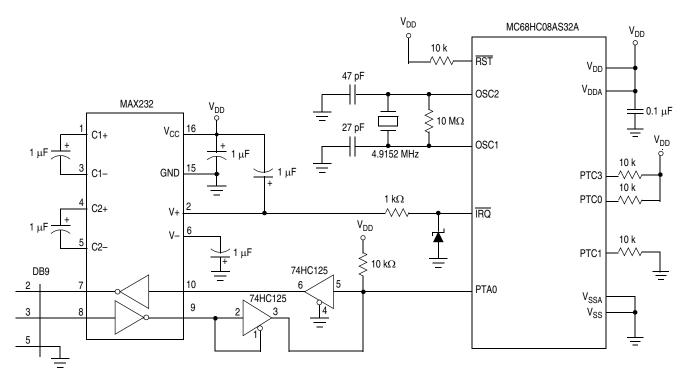
Figure 17-7. Normal Monitor Mode Circuit
