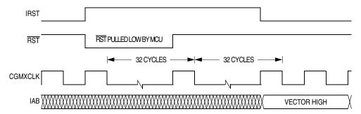
Figure 14-6. Internal Reset Timing
