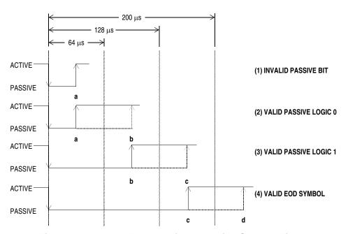
Figure 4-9. J1850 VPW Received Passive Symbol Times
