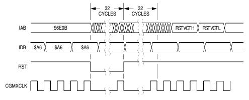
Figure 14-15. Wait Recovery from Internal Reset
