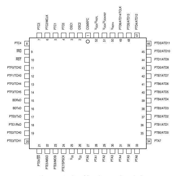
Figure 1-2. 52-Pin PLCC Assignments (Top View)
