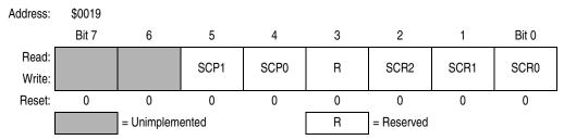
Figure 13-17. SCI Baud Rate Register (SCBR)
