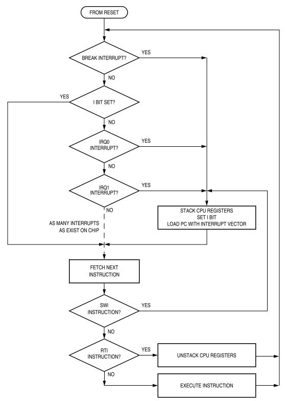
Figure 14-11. Interrupt Processing
