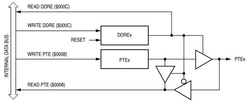
Figure 12-16. Port E I/O Circuit
