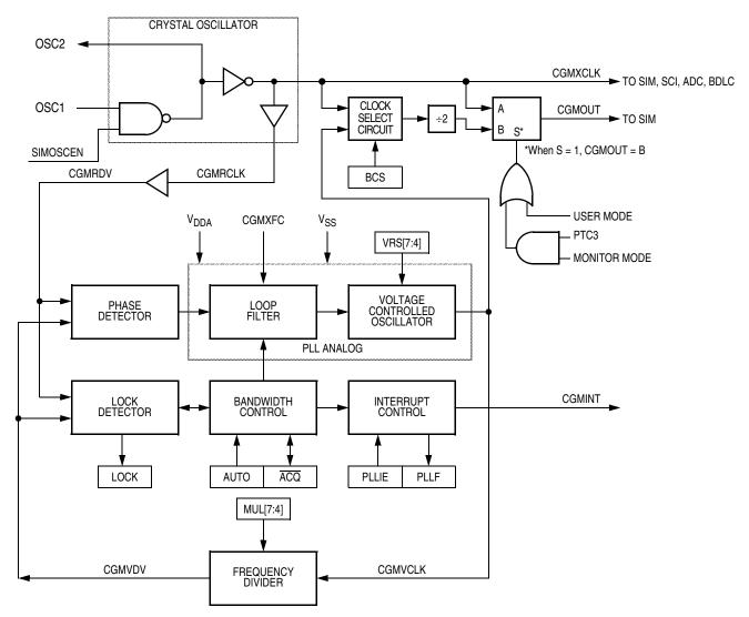
Figure 5-1. CGM Block Diagram
