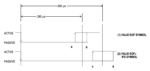
Figure 4-10. J1850 VPW Received Passive EOF and IFS Symbol Times
