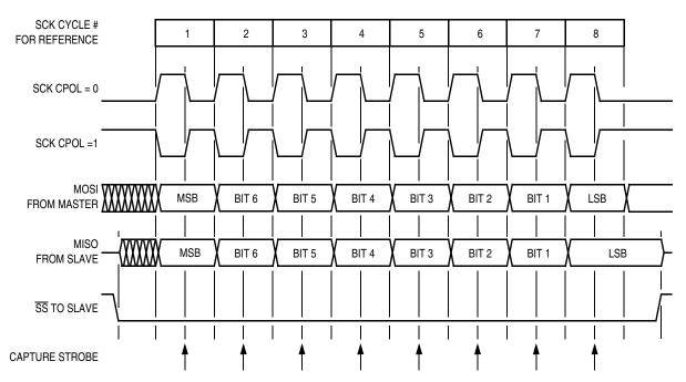
Figure 15-7. Transmission Format (CPHA = 1)
