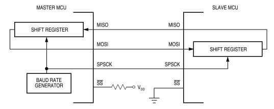
Figure 15-4. Full-Duplex Master-Slave Connections
