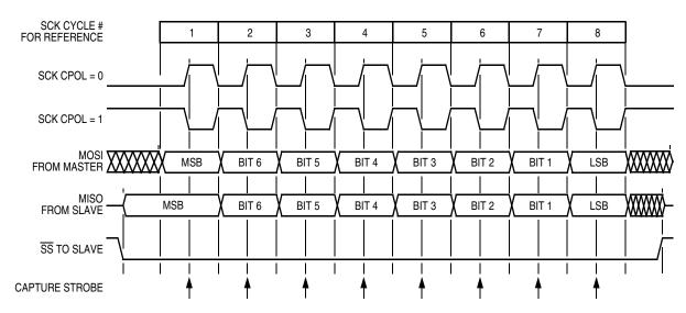
Figure 15-5. Transmission Format (CPHA = 0)
