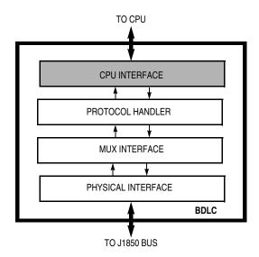
Figure 4-16. BDLC Block Diagram
