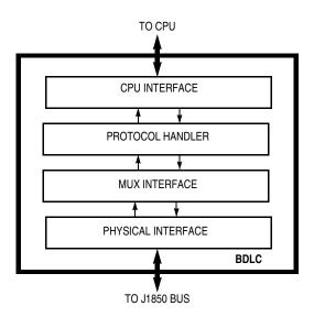
Figure 4-2. BDLC Block Diagram
