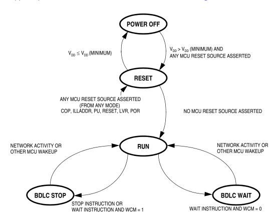
Figure 4-4. BDLC Operating Modes State Diagram
