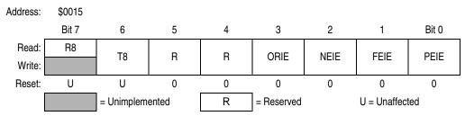
Figure 13-12. SCI Control Register 3 (SCC3)
