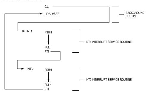
Figure 14-12. Interrupt Recognition Example
