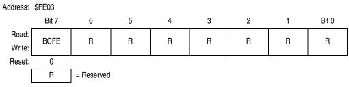
Figure 14-20. SIM Break Flag Control Register (SBFCR)
