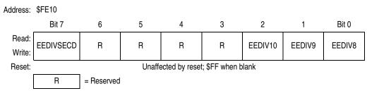
Figure 2-8. EEPROM Divider Non-Volatile Register High (EEDIVHNVR)
