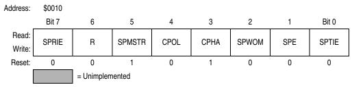
Figure 15-14. SPI Control Register (SPCR)
