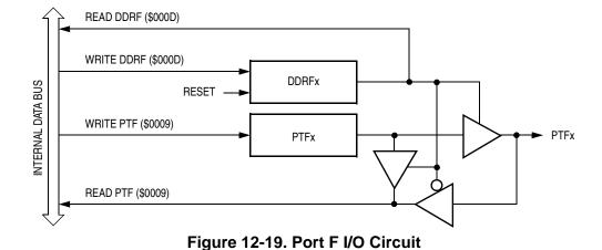
When bit DDRFx is a logic 1, reading address \$0009 reads the PTFx data latch. When bit DDRFx is a logic 0, reading address \$0009 reads the voltage level on the pin. The data latch can always be written, regardless of the state of its data direction bit. **Table 12-6** summarizes the operation of the port F pins.
