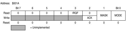
Figure 8-5. IRQ Status and Control Register (ISCR)
