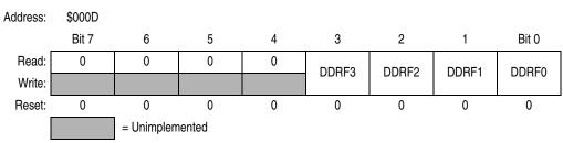
Figure 12-18. Data Direction Register F (DDRF)
