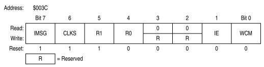
Figure 4-18. BDLC Control Register 1 (BCR1)
