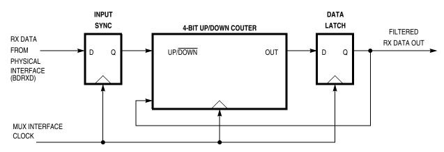
Figure 4-6. BDLC Rx Digital Filter Block Diagram
