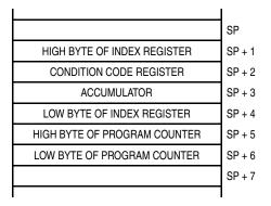
Figure 17-12. Stack Pointer at Monitor Mode Entry
