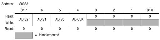
Figure 3-5. ADC Input Clock Register (ADICLK)
