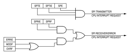
Figure 15-11. SPI Interrupt Request Generation
