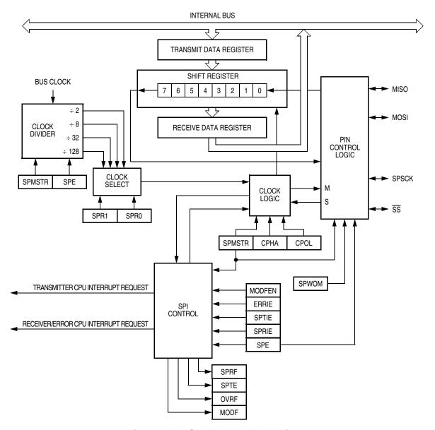
Figure 15-3. SPI Module Block Diagram
