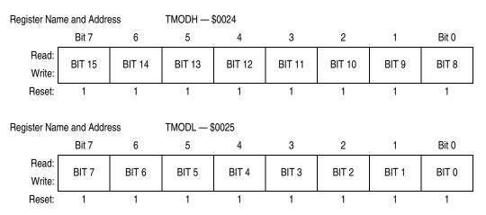
Figure 16-7. TIM Counter Modulo Registers (TMODH and TMODL)
