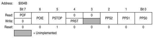
Figure 11-3. PIT Status and Control Register (PSC)
