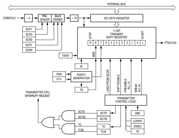
Figure 13-5. SCI Transmitter
