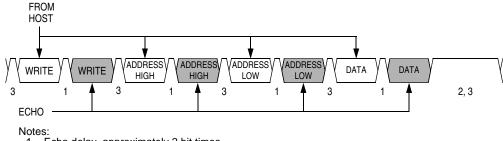
1 = Echo delay, approximately 2 bit times 2 = Cancel command delay, 11 bit times
