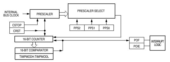
Figure 11-1. PIT Block Diagram
