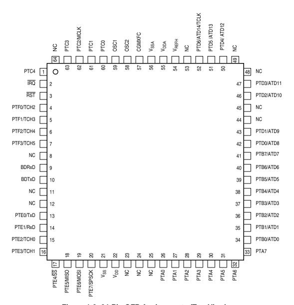
Figure 1-3. 64-Pin QFP Assignments (Top View)
