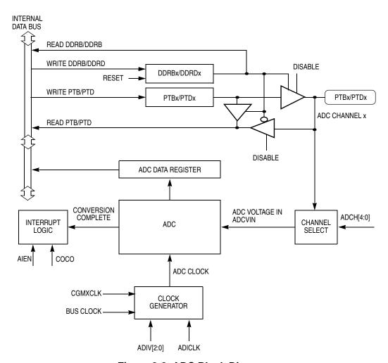
Figure 3-2. ADC Block Diagram
