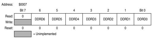
Figure 12-12. Data Direction Register D (DDRD)
