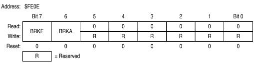
Figure 17-3. Break Status and Control Register (BRKSCR)
