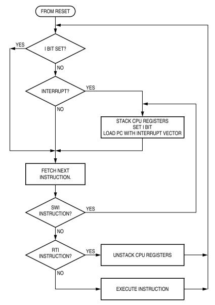
Figure 8-4. IRQ Interrupt Flowchart
