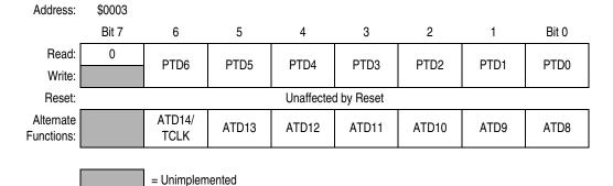
Figure 12-11. Port D Data Register (PTD)
