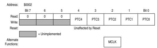
Figure 12-8. Port C Data Register (PTC)
