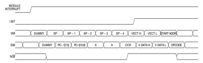
Figure 14-9. Hardware Interrupt Entry
