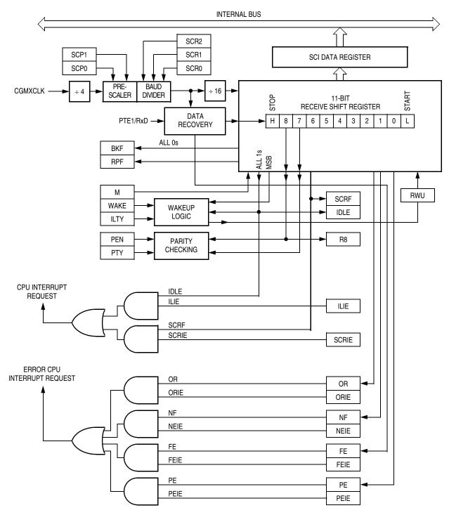
Figure 13-6. SCI Receiver Block Diagram
