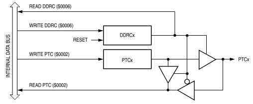
Figure 12-10. Port C I/O Circuit
