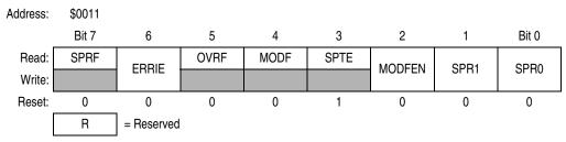
Figure 15-15. SPI Status and Control Register (SPSCR)
