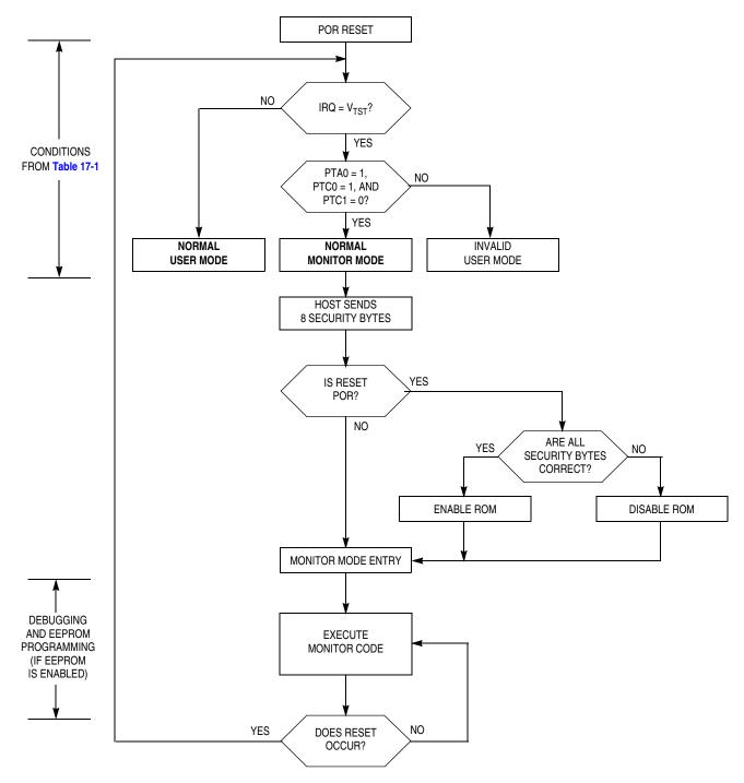
Figure 17-6. Simplified Monitor Mode Entry Flowchart
