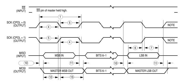
NOTE: This last clock edge is generated internally, but is not seen at the SCK pin.
