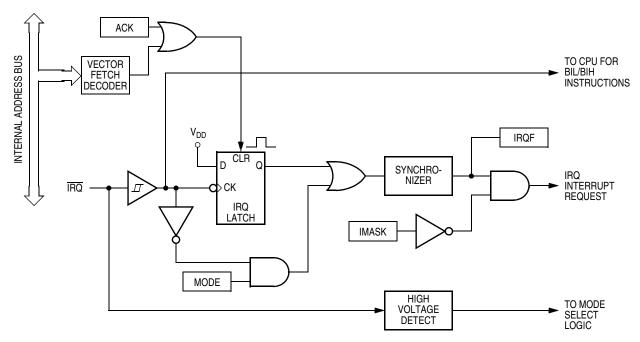
Figure 8-1. IRQ Block Diagram
